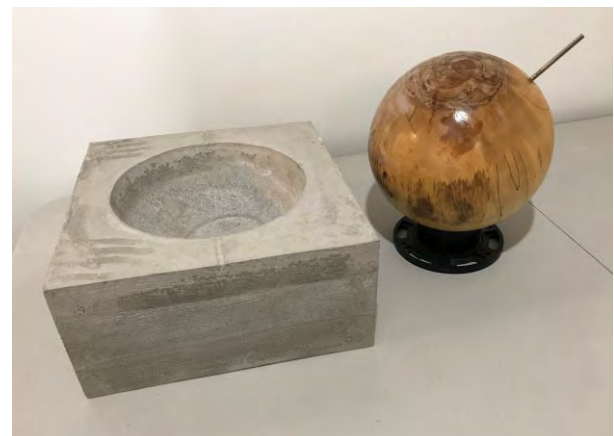
Figure 8: A gypsum - cement mold created as a negative mold from a wooden sphere made by a wood turner.
