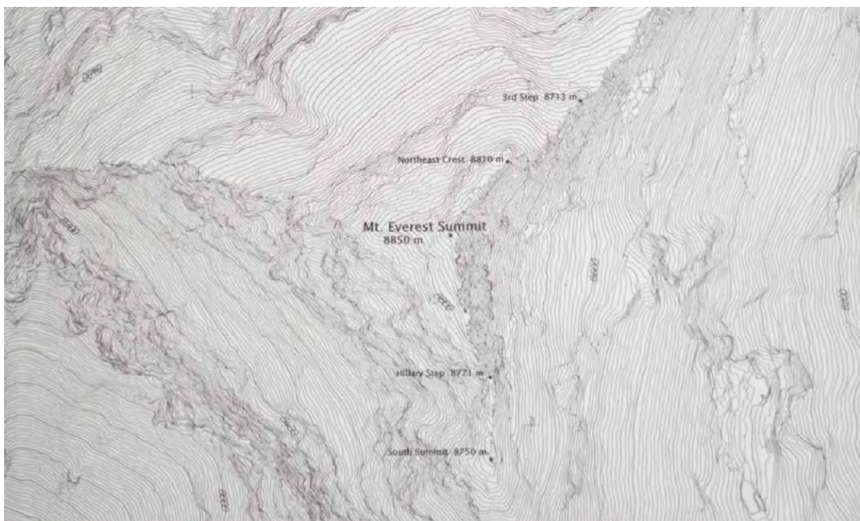
Figure 29: Map (c.2000) with 1 to 5000 contours derived from Washburn airphotos from the 1980s. This image is a portion of a display map from about 1999-2001 (source National Geographic Library).
