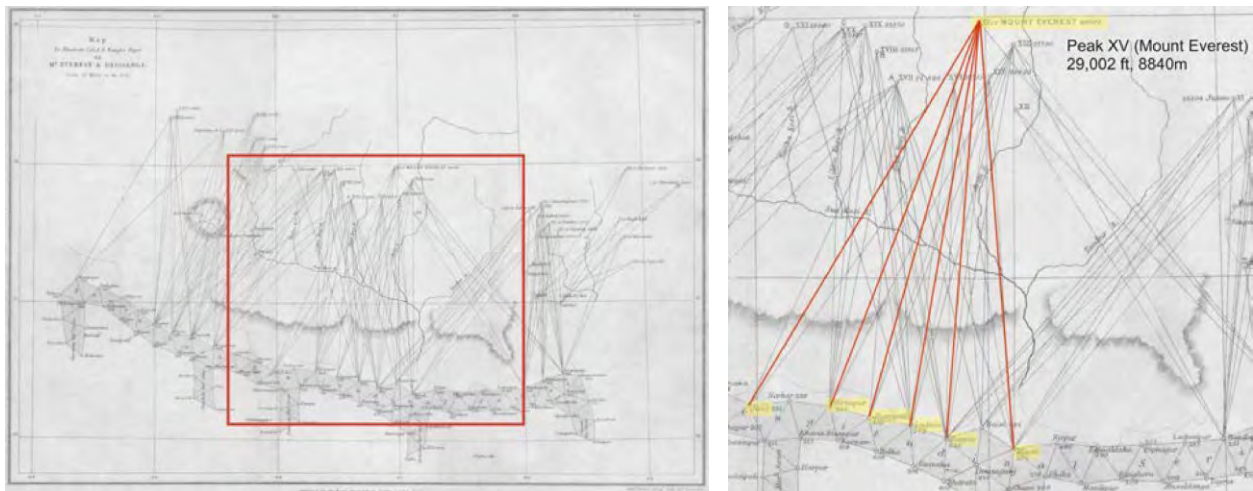
Figure 6: Andrew Waugh's illustration of the Survey of India's work to determine the height of Mount Everest (Waugh 1858). The work was based on surveys from 1849-1850.
