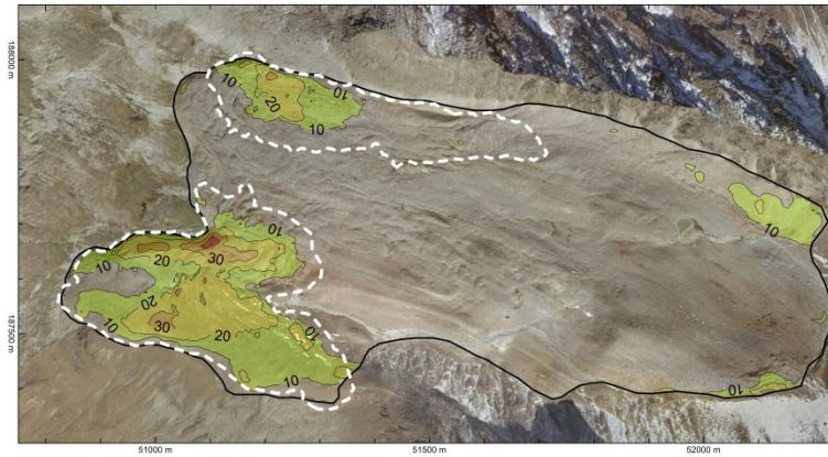
Figure 13: Mean annual horizontal flow velocity for the time period 2003-2010. Isotachs ( \text{cm a}^{-1} ), significance level at 10 \text{ cm a}^{-1} ( 3 \sigma ).
