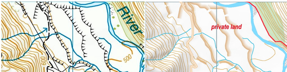
Figure 1: River terraces – left: traditional symbol (Topo50 sheet BU23 enlarged 185%), right: an alternative presentation (NewTopo Lake Sumner enlarged 140%).
