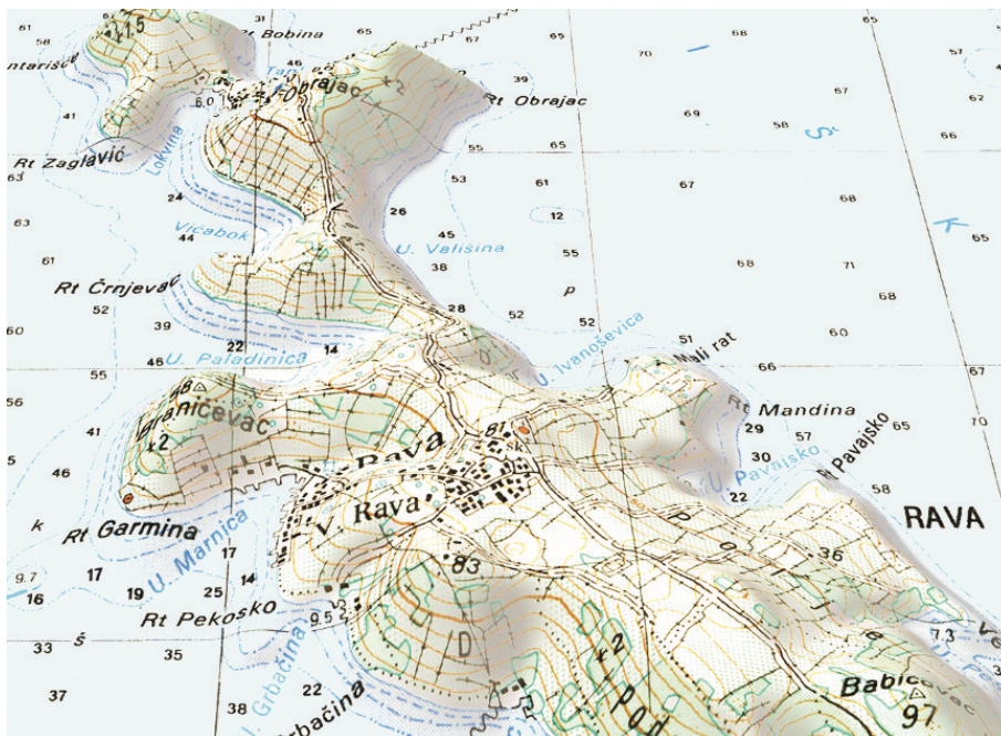
Figure 3: A DTM overlaid with a topographic map. The vector contours from the topographic map were used as input for DTM generation by interpolation similar to manual methods from maps (Kuveždić et al. 2008).
