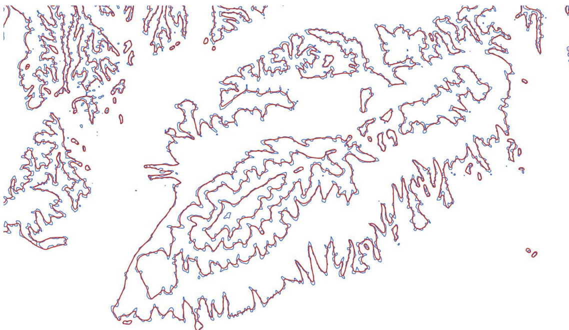
Figure 4: Contours generated from a DTM with resolution of 25 m (blue) and contours on a topographic map in the scale 1:500,000, manually generalised from a larger scale topographic map (red).
