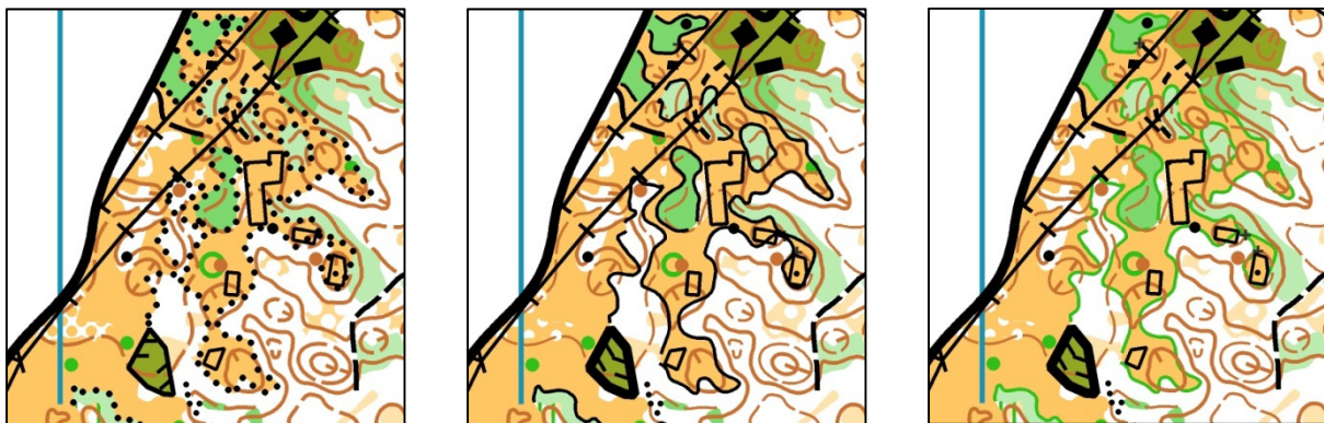
Figure 9: Three possible symbols for distinct vegetation boundary in ISOM 201x draft – map of Kalce, Slovenia, drawn by Matjaž Štanfel.
